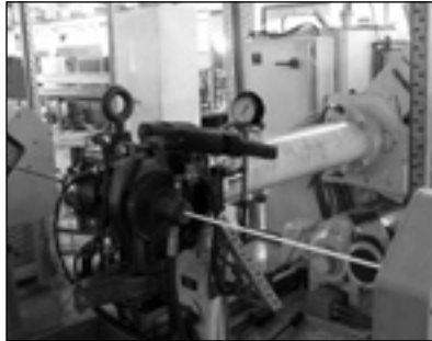
Pictured is a rubber hose coating line with a precision Model 2000 crosshead.
