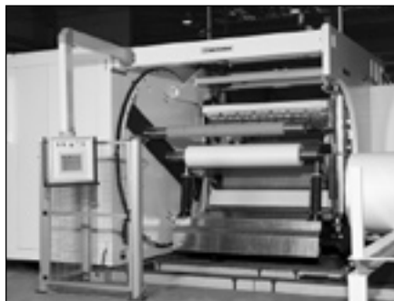
The new Culisse winder is engineered for high-speed in-line winding and slitting of extra wide film webs.
