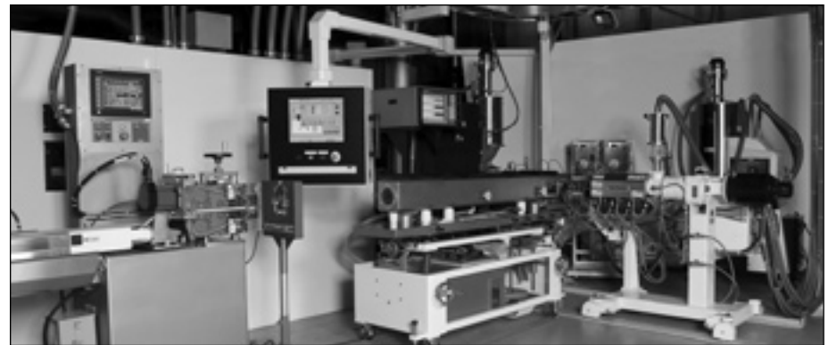
This medical tubing line at Davis-Standard's Pawcatuck facility is available for customer trials and testing.
