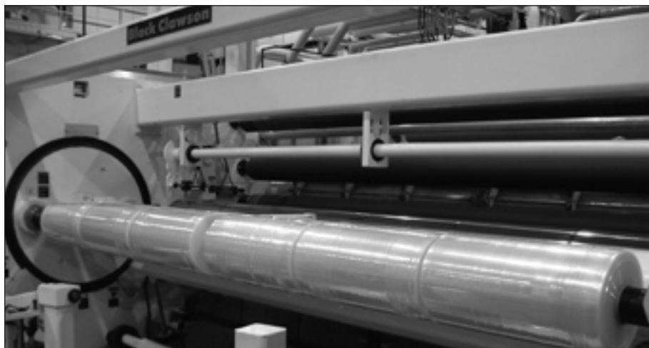
Intertape's new six-up stretch film line is used for producing standard and differential cling films at high speeds.
