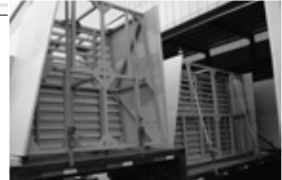
Modular gusset sections prepared for shipment.
