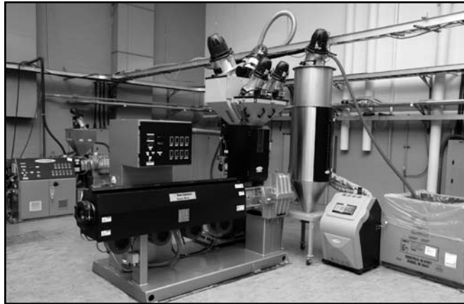
Conair uses its 3 1/2-inch (90mm) extruder to develop and test new downstream equipment.
