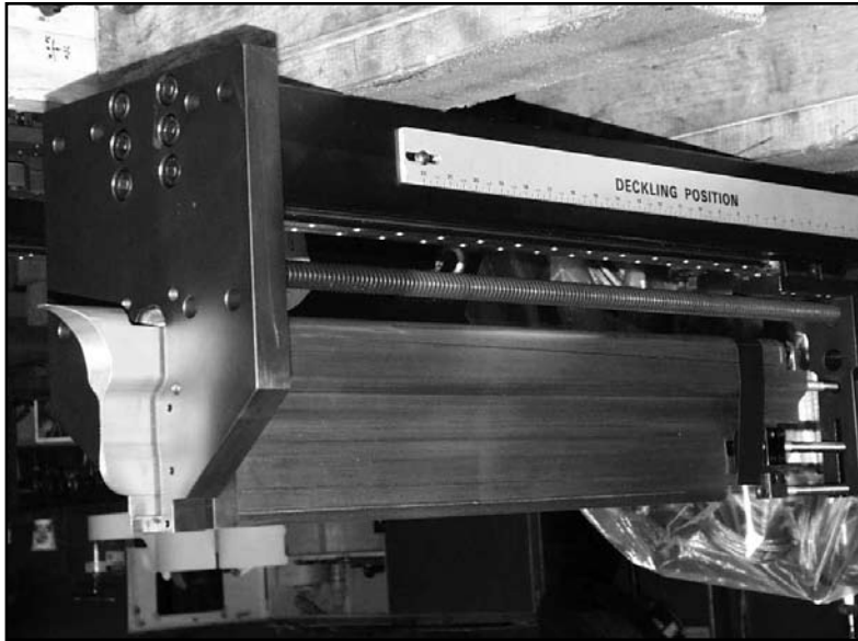
Advantages of the Series 50 include reduced edge bead, an internal deckle system and removable lips for die cleaning.
