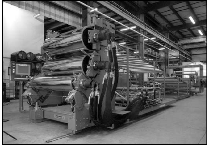
The XP Express™ can be configured in an upstack, downstack, offset top or offset bottom arrangement. Machine shown without guards to demonstrate features.
