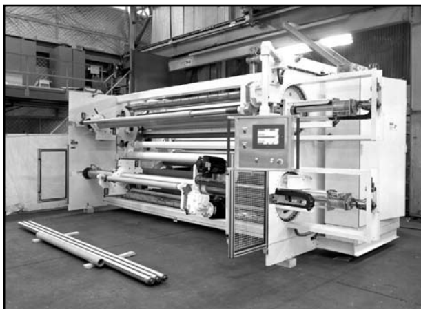
The Model 1650 winder is capable of winding film in widths up to 150 inches (3,810mm).
